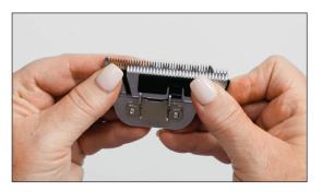
Remove Cutter Assembly for cleaning by sliding with your fingers to separate lower blade.
