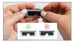
Attach Magnet Carrier to top of Cutter, not in cutter channel.
