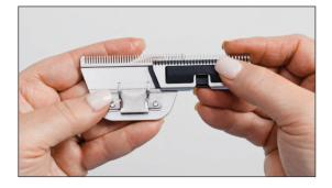
Slide assembly back into channel of the Lower Blade.
