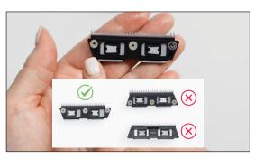
Place Bearing Cart back on assembly. Bearing Cart sides should match the same angle as the cutter angle and magnets should be by teeth of the cutter. You see 5 magnets - 3 circles & 2 rectangles as shown.
