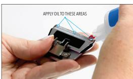
Apply oil by placing 3 drops along teeth of blade. Wipe off any excess oil.
