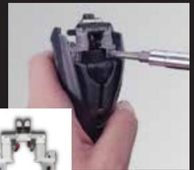
**HOW:** Turn off clipper and snap off the detachable blade. Slide off blade drive cap. Remove screws with a Phillips screwdriver and lift out drive assembly. Insert new blade drive and reverse steps to complete.
